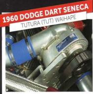
ENGINE: 318ci Mopar, 8:1 compression, forged pistons, H-beam rods, steel crank, remote oil filter system, ported heads, adjustable rockers, mild cam, 1370cfm FAST throttle body, FAST ECU, Procharger PISC supercharger, FAST dual sync distributor, MSD 6AL ignition, MSD Blaster coil, MSD leads, twin 2.5-inch exhaust, Flowmaster mufflers, custom alloy radiator, SPAL electric fan
