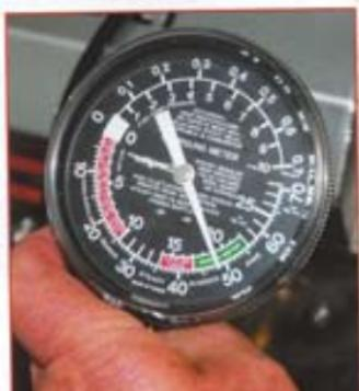
The idle circuits were neat up. Craig used a vacuum gauge to check where we were at. We'd set them too lean so he reset the idle mixture into the green zone with idle speed at 750 rpm. This had an immediate effect on the idle; it was much smoother.
